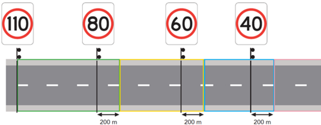
Figure 2.6: Appropriate speed use for sign placement
