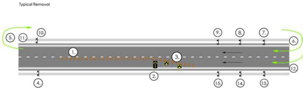
Figure 8.5: Multilane divided – typical removal sequence
